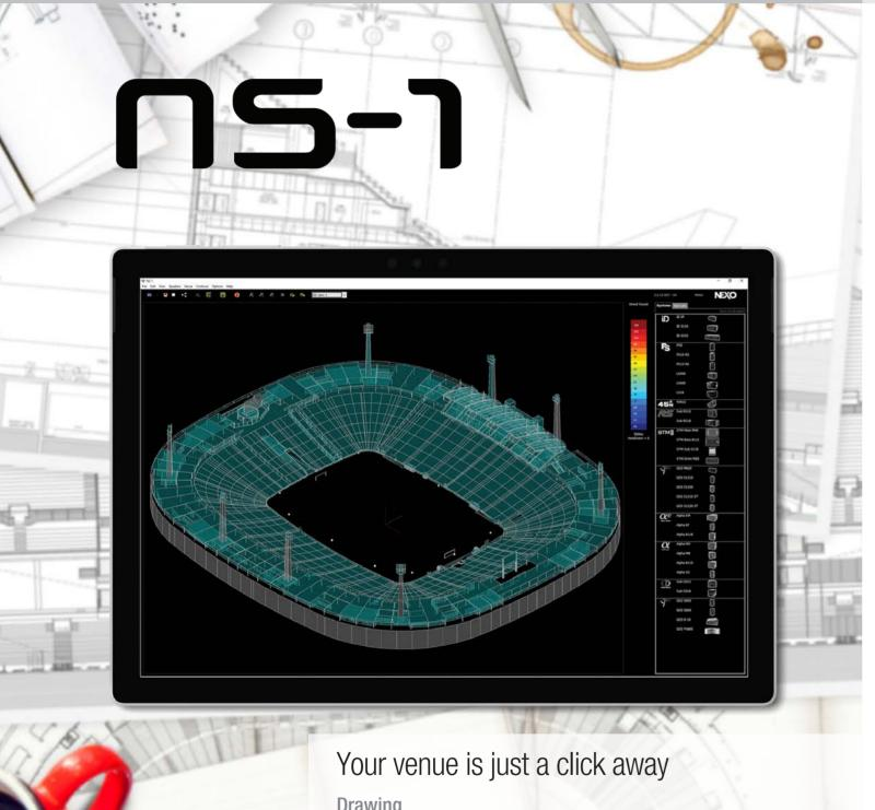
NS-1's drawing tools enable the user to design a venue very quickly. You can even import one or several images of 2D drawings such as plane or cross-section views, and design your 3D model accordingly.
