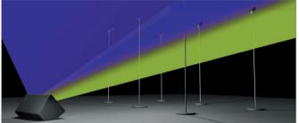
In conventional Front Of House configuration, a PS R2 Series loudspeaker yields 50° horizontal coverage at 25° above the centre line. Rotating the horn expands this to 100° at 50° below the centre line, such that coverage parrows
