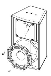
To access the HF diaphragm, remove the 4 screws. Tightening torque: 1.7 Nm
