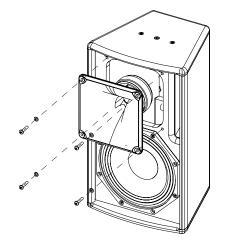
Reassemble the assembly and replace the grille.
