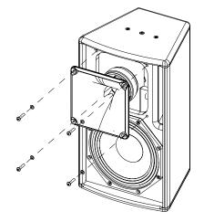
Reassemble the assembly and replace the grille.
