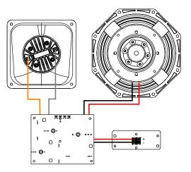
→ To wire ePS8, slit the membrane of the grommet crosswise, pass the cable through and make the connection to the screw terminals. Place the IPCOV.
