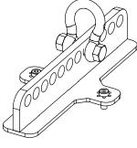
Remove 2 screws on the top Screw VNU-BUMP to ePS8 (use only screws provided with VNU-BUMP). Tight properly.
