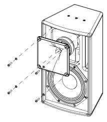
Reassemble the assembly and replace the grille.
