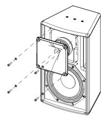
Position the horn according to the desired HF dispersion.
