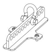
Remove 2 screws on the top Screw VNU-BUMP to ePS8-EN54 (use only screws provided with VNU-BUMP). Tight properly.
