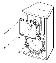
Reassemble the assembly and replace the grille.
