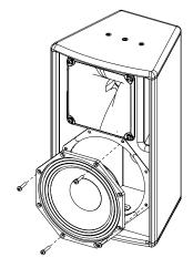
To access the HF diaphragm, remove the 4 screws. Tightening torque: 1.7 Nm
