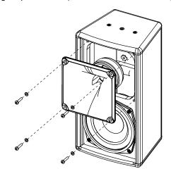
Reassemble the assembly and replace the grille.
