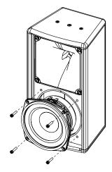
To access the HF diaphragm, remove the 4 screws.
