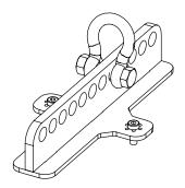
Remove 2 screws on the top Screw VNU-BUMP to ePS6 (use only screws provided with VNU-BUMP). Tight properly.
