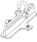
Remove 2 screws on the top Screw VNU-BUMP to ePS6 (use only screws provided with VNU-BUMP). Tight properly.
