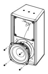
To access the HF diaphragm, remove the 4 screws. Tightening torque: 1.7 Nm
