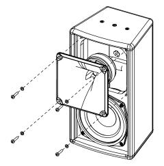
Reassemble the assembly and replace the grille.
