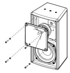
Reassemble the assembly and replace the grille.
