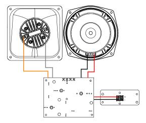
→ To wire ePS6, slit the membrane of the grommet crosswise, pass the cable through and make the connection to the screw terminals. Place the IPCOV.
