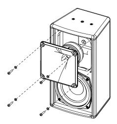
Position the horn according to the desired HF dispersion.
