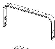
Remove the M10 inserts from each side. Place HBRK365 on ePS6, use only fasteners provided. Tight properly.
