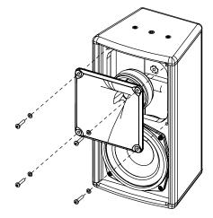
Reassemble the assembly and replace the grille.
