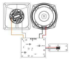
→ To wire ePS6-EN54, slit the membrane of the grommet crosswise, pass the cable through and make the connection to the screw terminals. Place the IPCOV.
