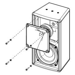
Reassemble the assembly and replace the grille.
