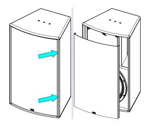
Remove the 4 screws at the back of ePS12 and the 4 screws that hold the horn. Remove it.
