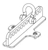
Remove 2 screws on the top Screw VNU-BUMP to ePS12 (use only screws provided with VNU-BUMP). Tight properly.
