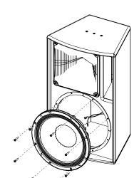
To access the HF diaphragm, remove the 4 screws. Tightening torque: 2.5 Nm
