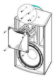
Reassemble the assembly and replace the grille.
