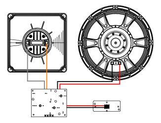
→ To wire ePS12, slit the membrane of the grommet crosswise, pass the cable through and make the connection to the screw terminals. Place the IPCOV.
