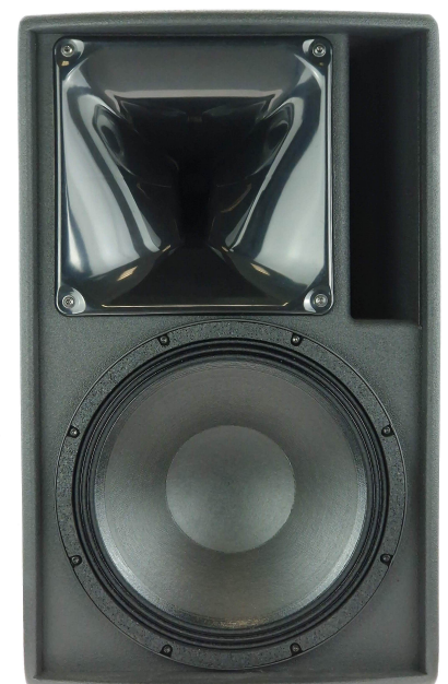
Grille removed, the large PS horn used with the HF driver
