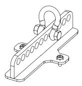
Remove 2 screws on the top Screw VNU-BUMP to ePS12-EN54 (use only screws provided with VNU-BUMP). Tight properly.
