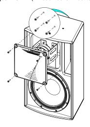
Reassemble the assembly and replace the grille.
