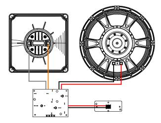
→ To wire ePS12-EN54, slit the membrane of the grommet crosswise, pass the cable through and make the connection to the screw terminals. Place the IPCOV.
