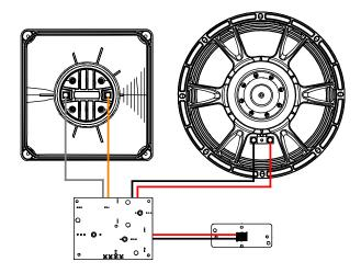
→ To wire ePS12-EN54, slit the membrane of the grommet crosswise, pass the cable through and make the connection to the screw terminals. Place the IPCOV.
