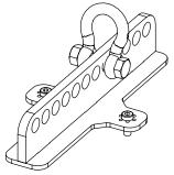
Remove 2 screws on the top Screw VNU-BUMP to ePS12-EN54 (use only screws provided with VNU-BUMP). Tight properly.
