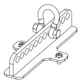
Remove 2 screws on the top Screw VNU-BUMP to ePS10 (use only screws provided with VNU-BUMP). Tight properly.
