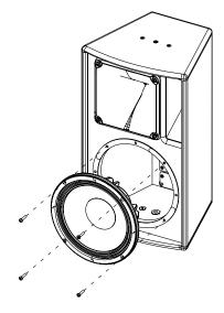
To access the HF diaphragm, remove the 4 screws. Tightening torque: 2.5 Nm
