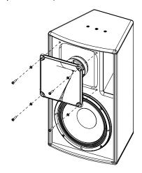
Reassemble the assembly and replace the grille.
