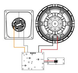
→ To wire ePS10, slit the membrane of the grommet crosswise, pass the cable through and make the connection to the screw terminals. Place the IPCOV.
