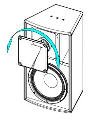
Reassemble the assembly and replace the grille.
