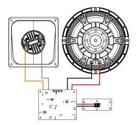
→ To wire ePS10, slit the membrane of the grommet crosswise, pass the cable through and make the connection to the screw terminals. Place the IPCOV.
