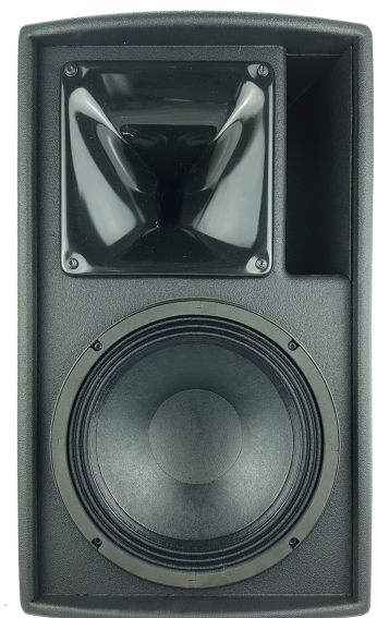
Grille removed, the large PS horn used with the HF driver
