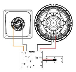
→ To wire ePS10-EN54, slit the membrane of the grommet crosswise, pass the cable through and make the connection to the screw terminals. Place the IPCOV.
