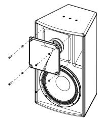
Reassemble the assembly and replace the grille.
