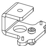
Screw VNI-CLADAPT to the ceiling (fasteners not provided).
