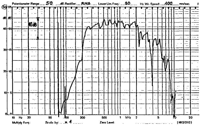
Fig 14 : detailed farfield on axis response, single midrange element, (unwarbled sine wave ). Zero level is 55 dB SPL at 4 meters with 4 Volts RMS on 8 Ohm nominal impedance (minimum impedance 9 Ohms) yielding a reference sensitivity of 107 dB/1 W/1 m.
