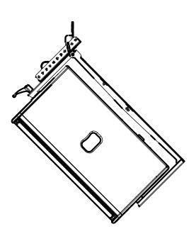
Adjust the angle with the different holes on VNT-TTC
