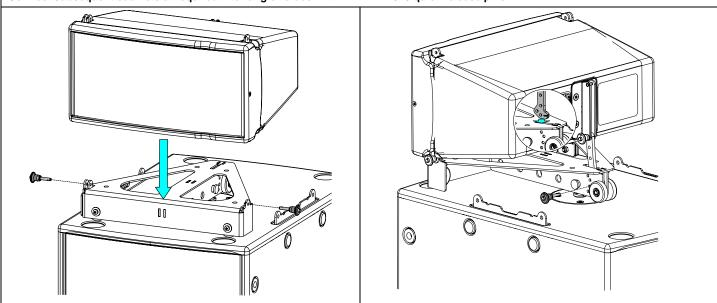
Ensure that the clevis pin is properly locked in VNT-MNSTKM6, and that 5mm pins are properly locked in GEO M6.
