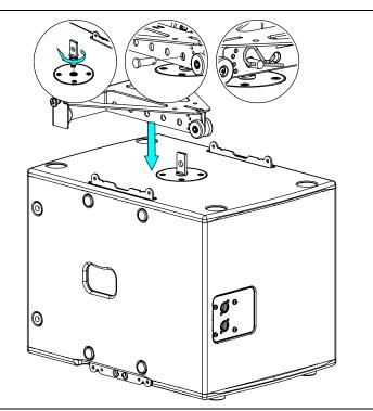
Connect bottom cabinet to GMT-BUMPER at required vertical angle with 4 x VXT-BL515 quick release pins NB: Bottom cabinet angle can be adjusted from -7° to 0° in relation to MSUB12.
