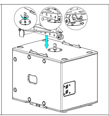
Connect bottom cabinet to GMT-BUMPER at required vertical angle with 4 x VXT-BL515 quick release pins NB: Bottom cabinet angle can be adjusted from -7 $^{\circ}$  to 0 $^{\circ}$  in relation to MSUB12.
