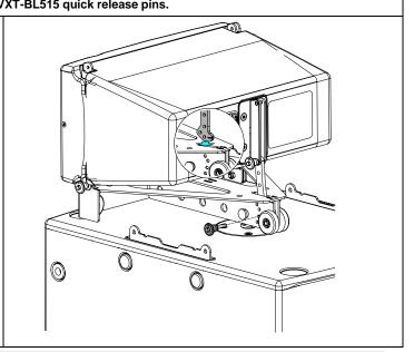
Ensure that the clevis pin is properly locked in VNT-MNSTKM6, and that 5mm pins are properly locked in GEO M6.
