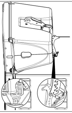
Adjust the angle between GEOM12 and MSUB18 using the Ball Lock of GEOM12 to lock the link bar of MNSTKM12 and GEOM12 (mark BUMPER and the desired angle).
