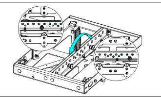
Place EXBARM6 by the top and fit the guides into the slots on the BUMPM6.
