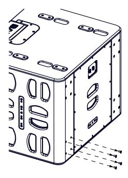
Fit the caster and secure it with the 4 notched screws supplied.
