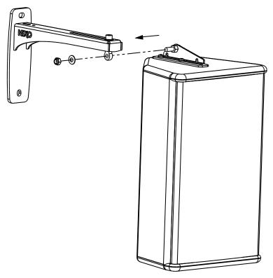
Tighten well to cancel any float between the arm and the adapter.
