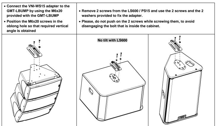
WARNING: Screws must be secured using Loctite 243<sup>™</sup>
