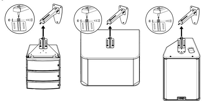
Tighten well to cancel any float between the arm and the adapter.
