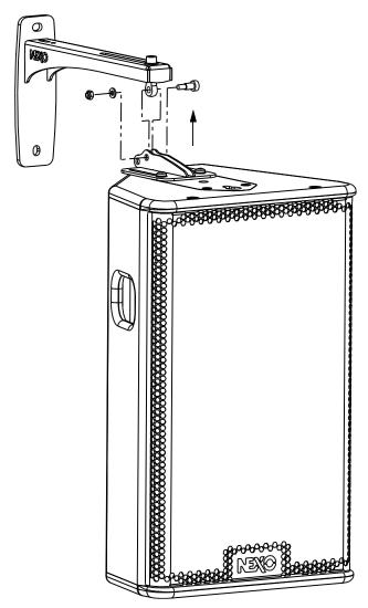
Tighten well to cancel any float between the arm and the adapter.
