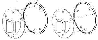
Place the speaker holder with NEXO Speaker into the wall bracket. Fix by tightening bolted assembly.
