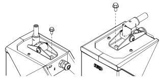
Use a 5mm ALLEN wrench for holding the tilt positions.
