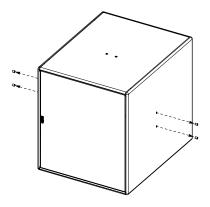
Place the assembly below the frame plate. Pay attention to the mounting direction, see the mark on the top frame. Fasten the M10x30 screws.
