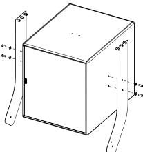
Remove the screws on both sides of ePS10.
