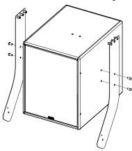
Remove the screws on both sides of ePS8.
