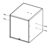
Assemble the Plates on each side of eLS400 using the M10x20 screws.
