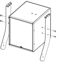
Place the assembly below the frame plate. Pay attention to the mounting direction, see the mark on the top frame.
