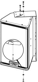
WARNING: Screws must be secured using Loctite 243<sup>™</sup>
