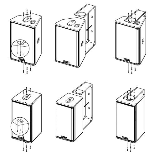
WARNING: Screws must be secured using Loctite 243™
