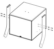
Place the assembly below the frame plate. Pay attention to the mounting direction, see the mark on the top frame.
