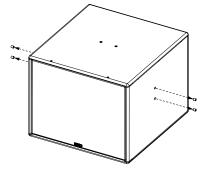
Place the assembly below the frame plate. Pay attention to the mounting direction, see the mark on the top frame. Fasten the M10x30 screws.
