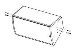
Remove the screws on both sides of ePS10.
