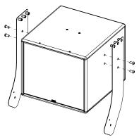
Remove the screws on both sides of ePS8.
