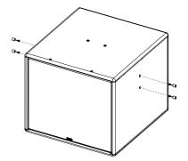
Place the assembly below the frame plate. Pay attention to the mounting direction, see the mark on the top frame. Fasten the M10x30 screws.
