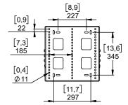
Ensure that the mounting location and fasteners can support at least 4 times the weight of all the installed cabinets, auxiliary equipment and cables.
