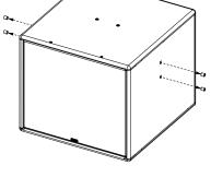
Remove the screws on both sides of ePS8.
