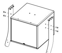
Assemble the Plates on each side of eLS400 using the M10x20
