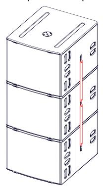
Speaker stand must always be installed on a horizontal surface.
