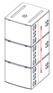
Speaker stand must always be installed on a horizontal surface. Stand height and footprint must be defined to prevent assembly from collapsing. Ensure that audience is not allowed within a safety area which radius is equal or higher than assembly height. Test steadiness of the assembly by pushing in all directions.
