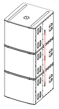
Speaker stand must always be installed on a horizontal surface. Stand height and footprint must be defined to prevent assembly from collapsing. Ensure that audience is not allowed within a safety area which radius is equal or higher than assembly height. Test steadiness of the assembly by pushing in all directions.
