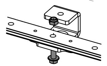
When L15 is up with HBRK15, position the fixing screw from below.
