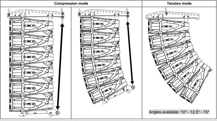
The force in the compression chain is limited to 750kg Use VXT-LEVA750
