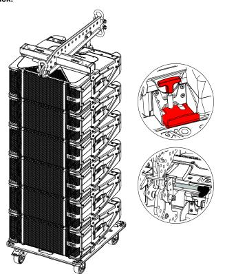
Side locking pins of LBUMPM28 must be flush to rigging plates on both sides of the cabinet. Ensure all RedLock<sup>™</sup> safety pins are locked into handle holes. Check rear quick release pins are fully engaged and locked.
