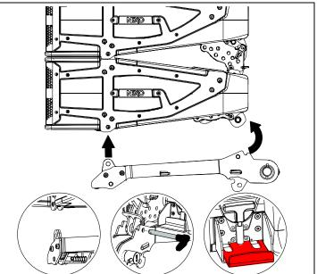
Ensure all RedLock<sup>™</sup> safety pins are locked into handle holes. Check rear quick release pins are fully engaged and locked.
